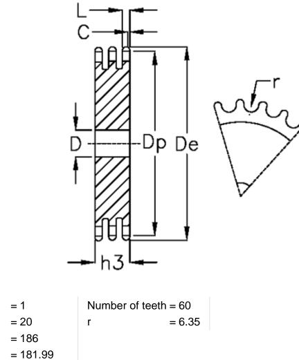
C = 1 D = 20 De = 186 Dp = 181.99 For chain size =  $3/8 \times 7/32$ For chain type = 06 B-3 h3 = 25.6 L = 5.2
